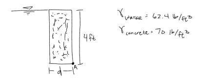
FIND RESULTANT HYDROSTATIC FORLE -> FIND THE TOTAL WEIGHT OF CONCRETE -> TAKE A MOMENT ABOUT POINT A -> SOLVE FOR "J"
